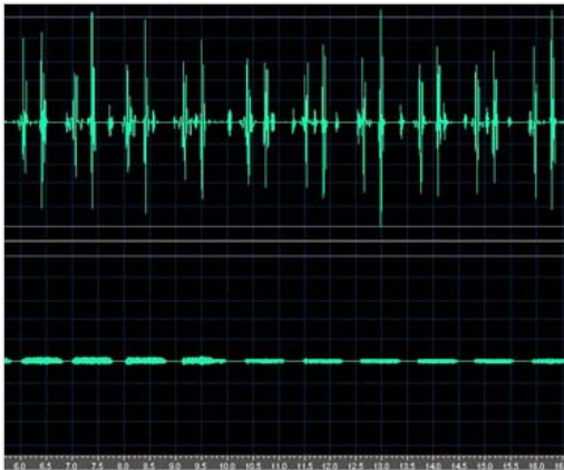
Separating and filtering structural and heart sounds (20-40 Hz) from scanner acoustic noise (>100 dB) enables OptiRhythm to produce very accurate gating.
